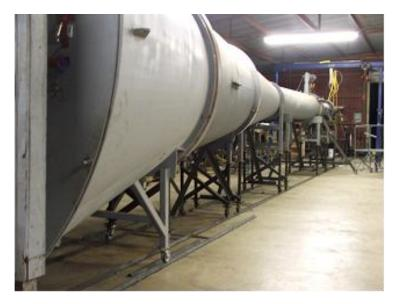
Figure 1. ABS Consulting Shock Tube Apparatus
