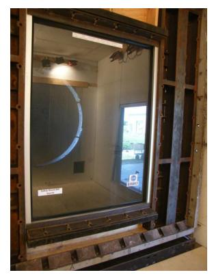
Figure 2. Window Mounted in Test Fixture
