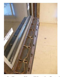
Figure 3. Close-up View of Mounting Restraints
