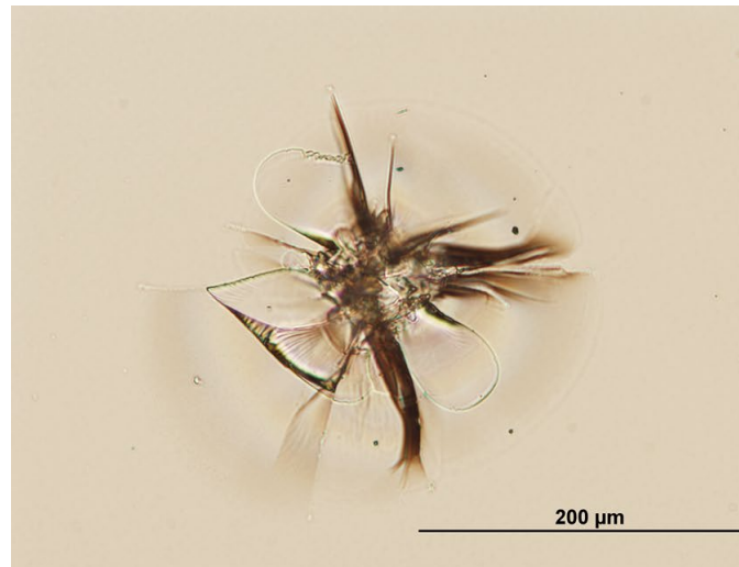
Untreated Glass Defect
